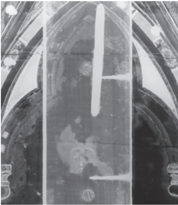
Fig. 2 X-radiograph of ironwork in the oak panels of the Retable. Image: The Dean and Chapter, Westminster Abbey.
