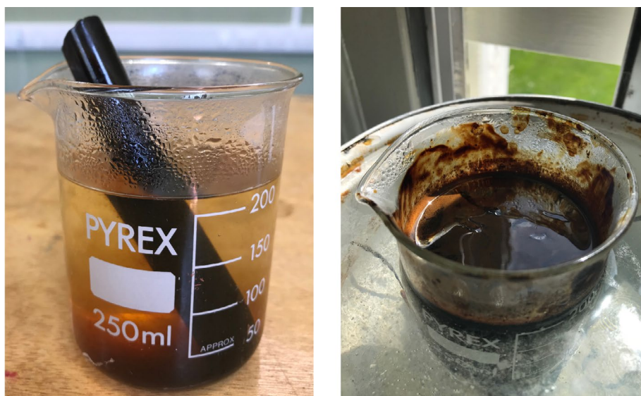
Figure 8. The preparation of the liquorice varnish, using liquorice sticks, heated and stored in a glass container. Left: Liquorice sticks in water prior to dissolution. Right: After dissolution. Photographs © Joanna Neville, Hamilton Kerr Institute, University of Cambridge.
