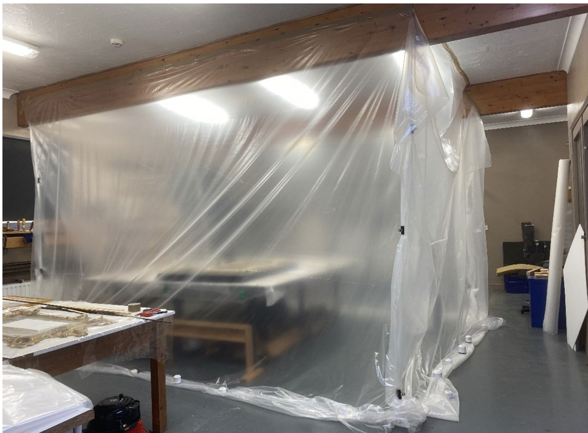
Figure 21. Humidity chamber constructed in the HKI studio, June–July 2023. Constructed and photographed by Alice Limb © Hamilton Kerr Institute, University of Cambridge.
