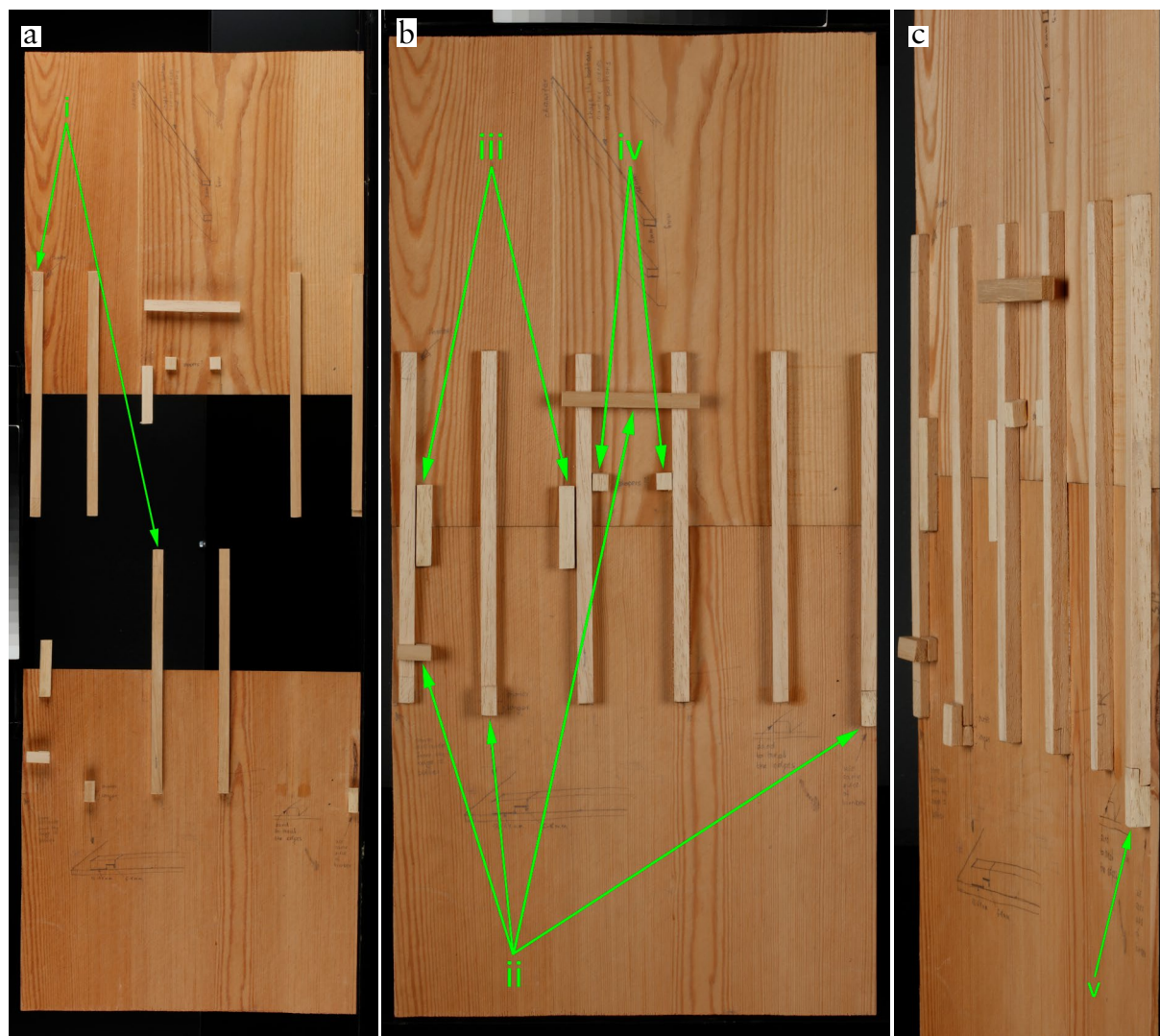
Figure 6. Mockup for joining the boards (a) showing (i) interlocking strips of wood, (b) showing (ii) different methods to block the strips of wood from collapsing, (iii) further strips of wood additionally adjusting the alignment of the boards, (iv) stoppers, (c) showing (v) chosen blocking method. Photographs © Justyna Kędziora, Hamilton Kerr Institute, University of Cambridge.
